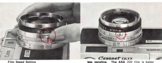
Immediately after loading film, be sure to set the ASA film speed scale in the proper position by pressing the notched film speed setting lever with your fingernail, matching the proper film speed number with the index of the ASA film speed indicator window.
